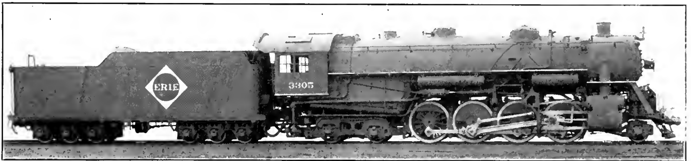
New 2-8-4 Type Locomotive of the Erie Railroad—Built by the American Locomotive Company
